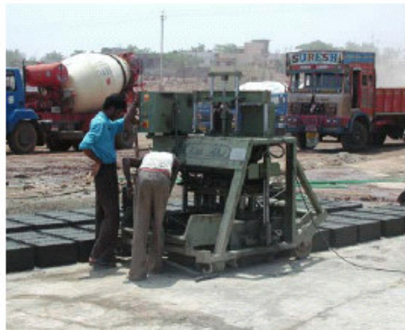
Fig 1. A&B: Akshay colony. C: Ready-mixed concrete plant of Suresh Enterprises in Hubli. D: Ready-mixed concrete trucks. E & F. Dry concrete and machinery used in the manufacture of large foundation blocks.
